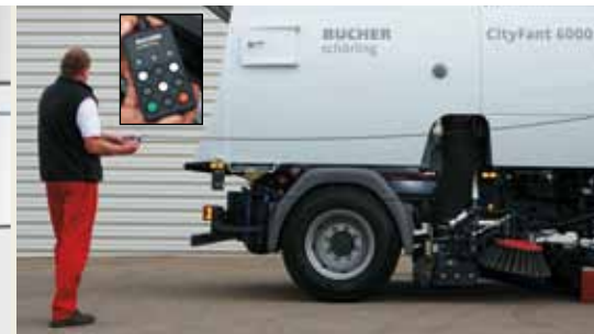
Hopper control unit
