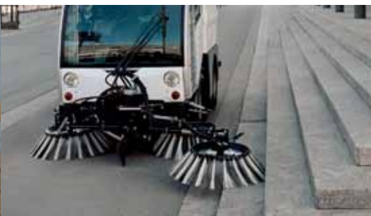
Fully adjustable front brush
